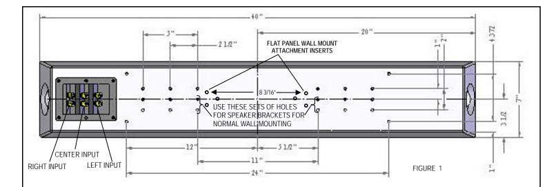
least 2 holes on each bracket that line up over a wall stud. Drill the wall and install your anchors and fasten the brackets to the wall with the "J" bend at the bottom (fig. 2 & 3).
